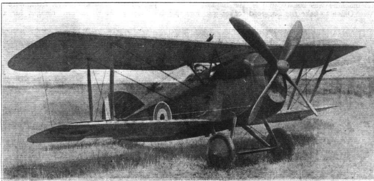
THE VICKERS F.B. 16 D. —The engine is a 150 h.p. Hispano-Suiza
